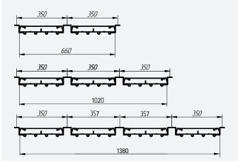
The thrust plate is bolted to the ceiling structures, which makes it possible to install Ecoterm Pro radiating ceiling panels close to the ceiling.
