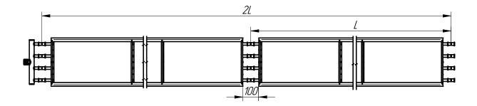
The panels can be connected in series to form a structure of almost any required length. In case of series connection, the steel pipes of the water circuit are connected using press fittings, supplied as optional equipment, all of which is discussed when placing the order.
