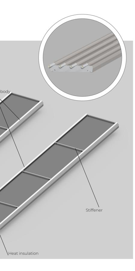
An additional feature distinguishing the Ecoterm Pro radiating ceiling panels from their analogues is the extra stiffeners necessary to protect the panel body, which is suspended from several points, from temporary deformation, such as "sagging", which can negatively affect the appliance's efficiency.
